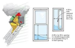
However, a 3<sup>rd</sup> floor attic space altered into a habitable bedroom or a basement bedroom must meet the currently adopted building code requirements for emergency escape openings.
